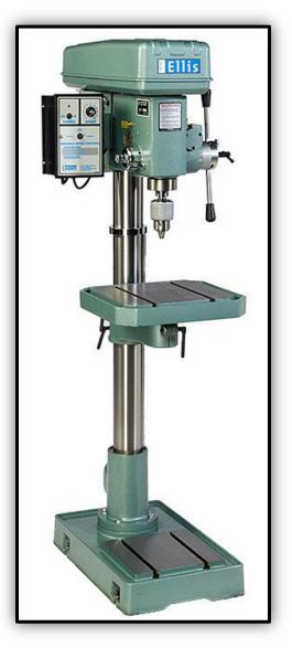
The drill press can be used with wood, aluminum and nylon. If you would like to drill other materials, please ask a mentor about how to do so safely. If you experience any problems while using the drill press such as grabbing, be sure to turn off the drill and ask for help. After drilling metal pieces please use the deburring tool to make the edges of the holes smooth. When using a hole saw drill bit, be sure that material does not get stuck in the bit.
